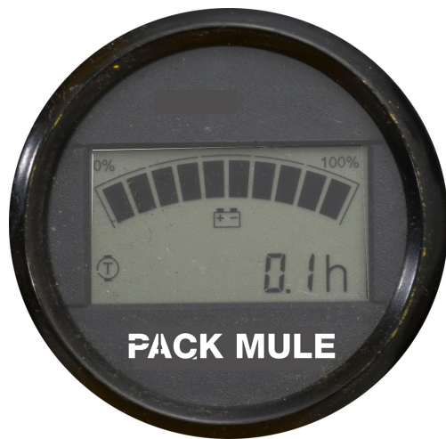
Figure 7: The Smart View Display, showing the battery state of charge and the current traction hours. If the system detects a fault, the display will show the fault code.
