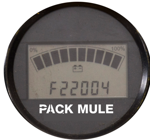
Figure 18: The Smart View display indicating a fault.
