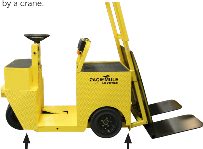
Figure 13: Position the jacks or jack stands indicated by arrows.
