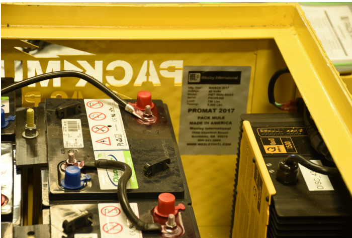
Figure 2: The Vehicle Identification Plate is located on the inside of the motor compartment. Please refer to this information when requesting warranty service, ordering replacement parts, or requesting service support from Wesley International.
